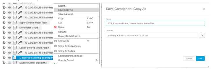
Go to the folder "Fusion 360/Machining/Sheets" and find the sheet with the right prefix (usually A6 or PC) that has the lowest letter designator that will fit your part(s). For example, if both A6.250a and A6.250b have room for your part, choose sheet A6.250a. In this case, it looks like A6.250b has room.
