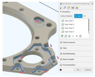
For blind (partial depth) operations, it is necessary to select the proper bottom height for this operation. Change the bottom height to be from "Selected Contours" and ensure 0 offset as shown.
