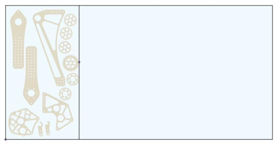
Drag the new part(s) into the sheet file, then use the "Arrange" tool with the settings shown. TIP: Drag the arrange tool from the dropdown menu up to the Toolbar so it's more accessible. If you don't you'll have to open the "MODIFY" dropdown menu to select the tool.
