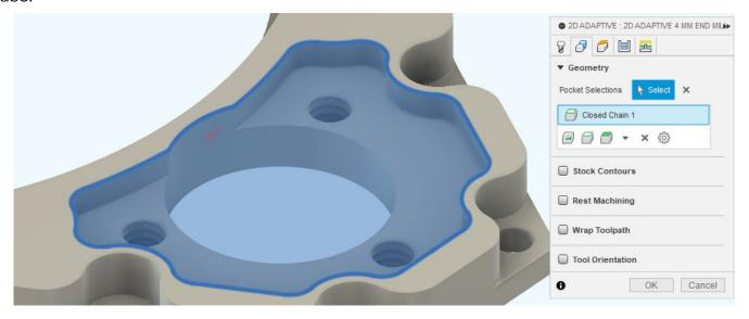
For blind (partial depth) operations, it is necessary to select the proper bottom height for this operation. Change the bottom height to be from "Selection", then select the face and ensure 0 offset as shown.
