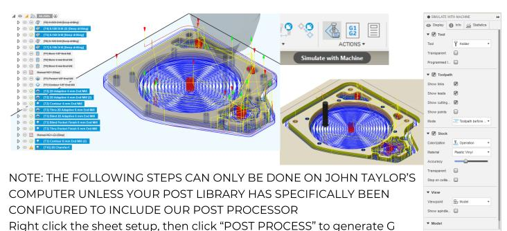
codes. Ensure settings are *identical* to what's shown below besides the "Name/number", "File name", and "Output folder" before posting. Overwrite the file if prompted. You will damage the machine if you don't take care during this step of the process. For example, "useG28" will make the spindle launch to a point that is likely not even on the machine between each operation, causing stalling, crashes, and other issues.
