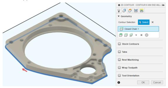
For **2D Chamfer** operations, click the "X" next to the selection box to clear any existing selections, then select any edges that can be chamfered to reduce the need to deburr the finished part. Blind pocket top edges in particular should be selected.
